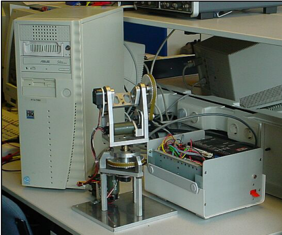
Figure 6 Photo of the JIWIY robotic set up and its controller box
