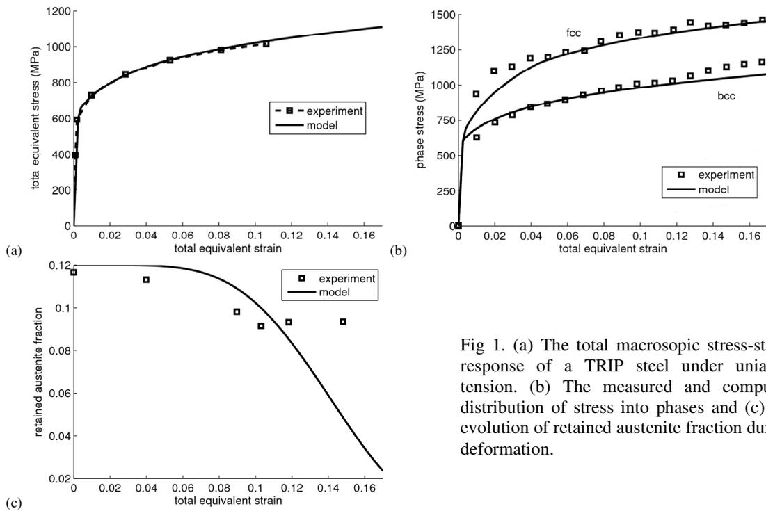
Fig 1. (a) The total macroscopic stress-strain response of a TRIP steel under uniaxial tension. (b) The measured and computed distribution of stress into phases and (c) the evolution of retained austenite fraction during deformation.
