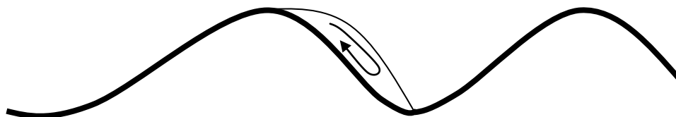
Figure 1 Schematization of the flow separation zone (flow from left to right)
