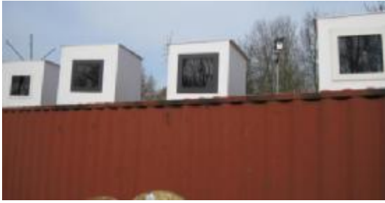
Figure 5 : The four test boxes on top of a sea container, after the third one a weather station is visible
