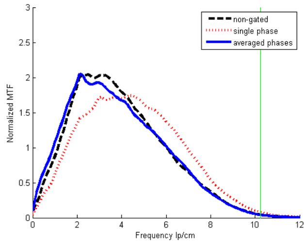
**Figure 3** – Illustration of the Modulation Transfer Function (MTF) of each dataset. The straight vertical line indicates the Nyquist frequency.
