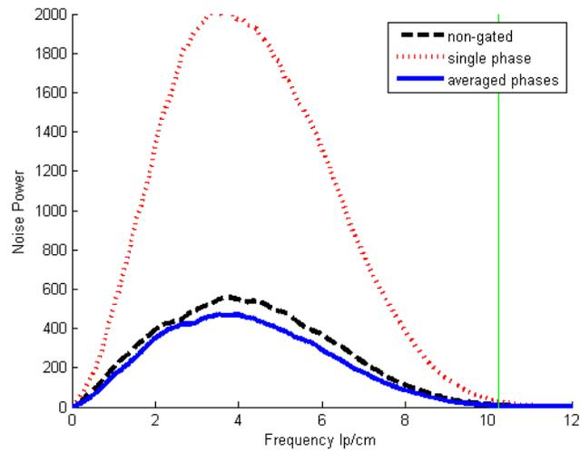
**Figure 2** – Illustration of the Noise Power Spectrum (NPS) of each dataset. The straight vertical line indicates the Nyquist frequency.
