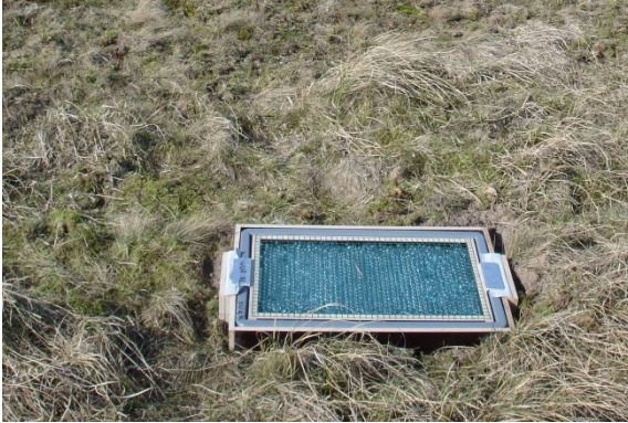
Figure 4. MDCO sediment trap for vertical sand deposition.
