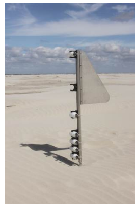
Figure 3. Sediment catcher on the beach of Ameland.
