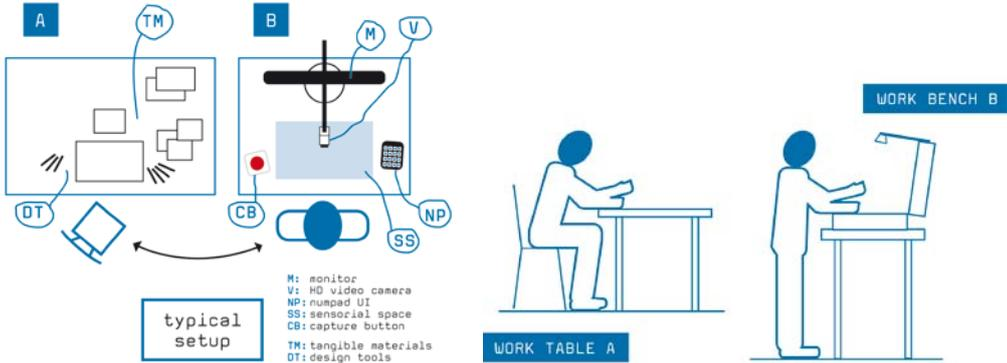
Figure 10. Typical setup experiment and multi-modal interaction - Design Ideation II.
