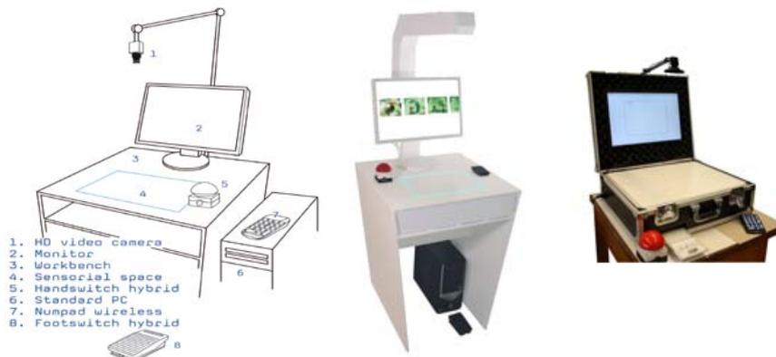
**Figure 5. LFDS workbench and flight-case setup.**
