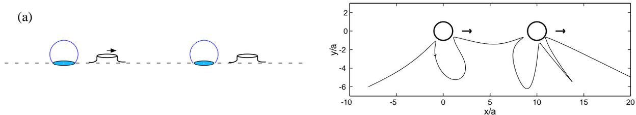
**Figure 2.** (a) Schematic structural elements for a microfluidic device: solid bumps are placed near the bubbles to direct the flow. (b) Predicted streaming.
