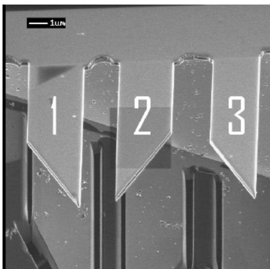
Figure 3. Three plane nanoneedles, marked with 1, 2, and 3. Below the nanoneedles, in the silicon bottom of the well, dicing lines are visible, produced during focused ion beam cutting of the sharp needle shape. Needle dimensions: 260 nm high, 3 μm wide and 10 μm long.
