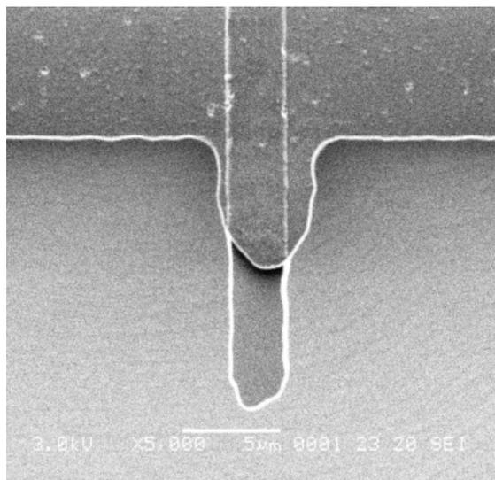
Figure 2. SEM-picture of an electrode needle. The electrode tip is 2 μm long, 2 μm wide and 100 nm high. Needle dimensions as in Figure 1.
