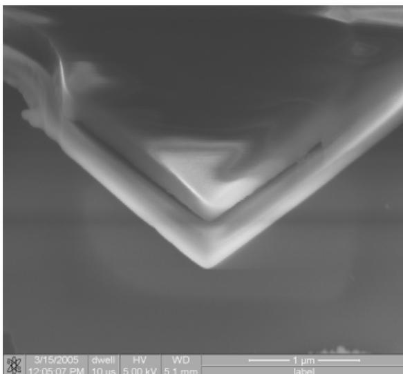
Figure 1. SEM-picture of a hollow nanoneedle. The channel is clearly visible in the middle of the needle. Inner channel dimensions: 150 nm high, 2 μm wide. Needle dimensions: 0.7 μm high, 3 μm wide and 5 μm long. The needle is sharpened by focused ion beam etching.
