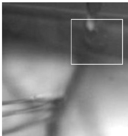
Figure 4. Microscopic picture of a HL60-cell punctured by a nanoneedle. The cell is positioned in the middle of the white square; the needle tip is the white tip in the top of the white square. In the lower left corner the external micropipette is shown.
