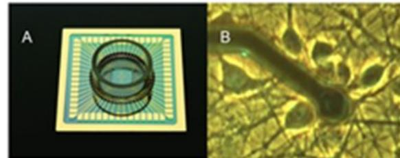
Figure 1. Multi electrode array (MEA) and close up of one of the electrodes. **A:** MEA, used to record neuronal activity in cultured cortical networks. It is based on a glass substrate with 60 embedded electrodes in the centre of the chamber, with 200 µm inter electrode distance. The glass ring glued on top was filled with glia conditioned growth medium and firmly sealed. **B:** close up of one of the electrodes and several neurons.
