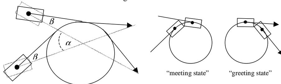
**Fig. 3.** Time optimal avoidance detour over equal distances.
