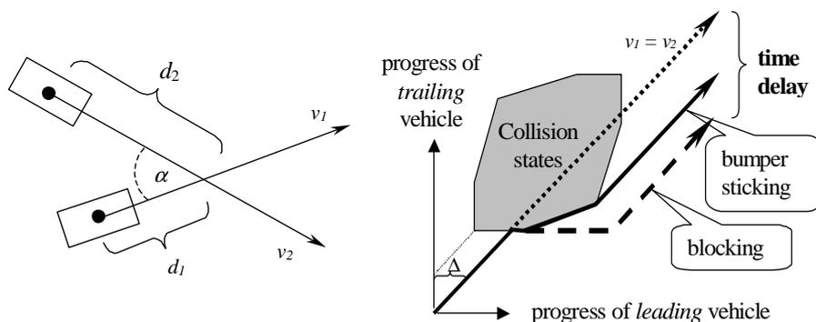
**Fig. 1.** Joint motion state diagram (shown on the right) of two vehicles crossing with angle  $\alpha$  (as shown on the left) with the leading vehicle having advantage  $\Delta = d_2 - d_1$  and the trailing vehicle adjusting its speed ( $v_2 \leq v_1$ ).
