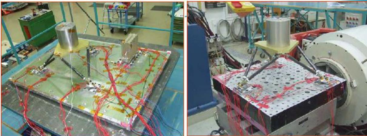
Figure 2: IFLV total and MIRI test setup on shaker slip table, courtesy [7]
