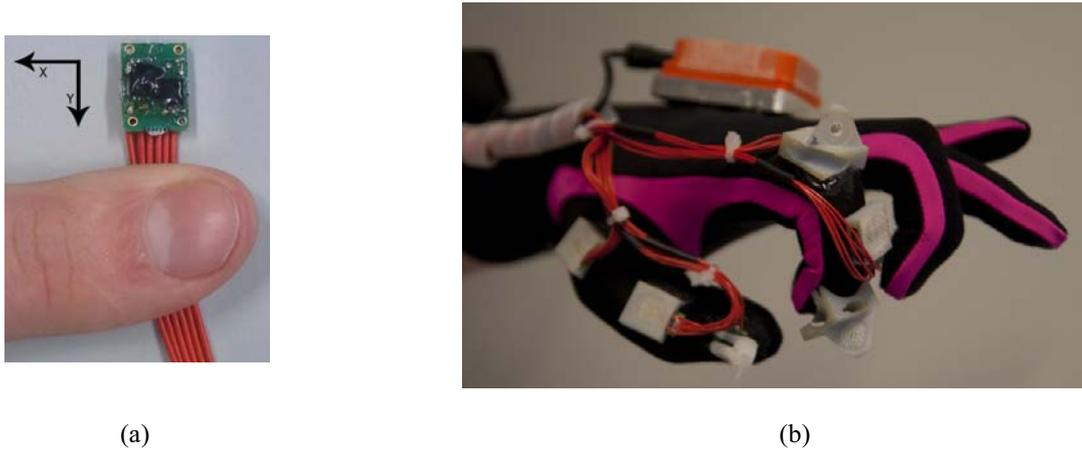
Figure 3. (a) Single sensor PCB containing a 3D accelerometer and 3D magnetometer (b) Instrumented glove. The PCB's are mounted in a synthetic housing (white). These sensor housings can be expanded with markers for optical measurements. In addition a full 3D IMU (orange, back of the hand is visible). The subject repeatedly made contact with the tips of index finger and thumb (pinch task).
