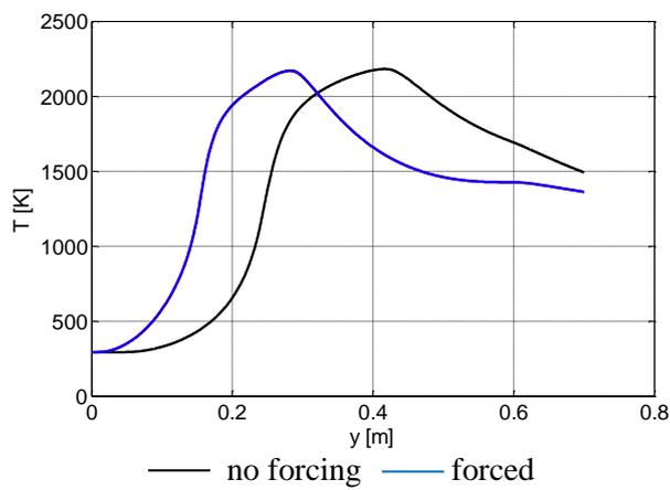
**Figure 5.5.** Time averaged temperature along the axial coordinate,  $x=3$  mm.
