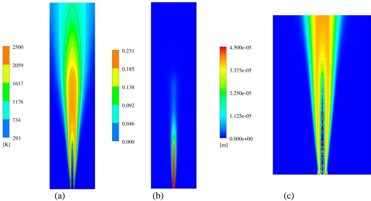
**Figure 5.1.** Instantaneous temperature (a),  $C_2H_6O$  mass fraction (b), liquid droplets diameter (c), at  $t=20ms$ .
