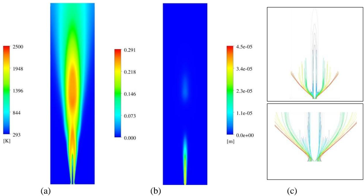
**Figure 5.6.** Instantaneous temperature (a),  $C_2H_6O$  mass fraction (b), liquid droplets diameter over gas fuel contours (grey lines) (c), at  $t=20$ ms. Acoustic forcing = 1500 Hz.
