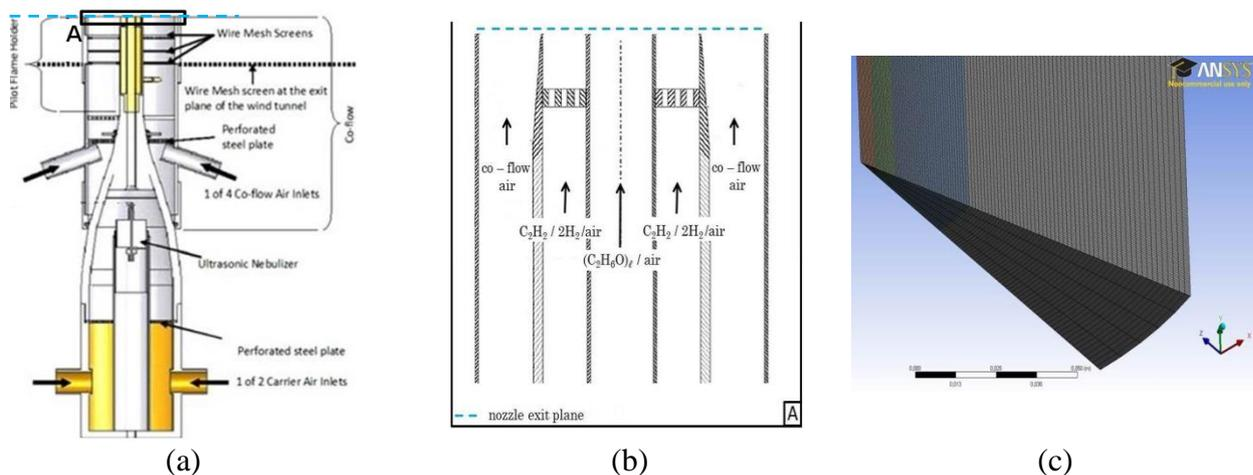
**Figure 2.1.** Schematic of the spray burner<sup>1</sup> (a), detail of the nozzle at the exit plane ( - ) (b), detail of the computational grid domain (c),
