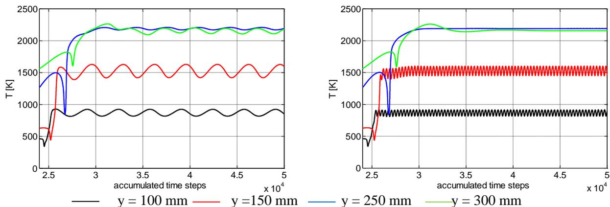
**Figure 5.3.** Instantaneous temperature: 150 Hz (left), 1500 Hz (right).
