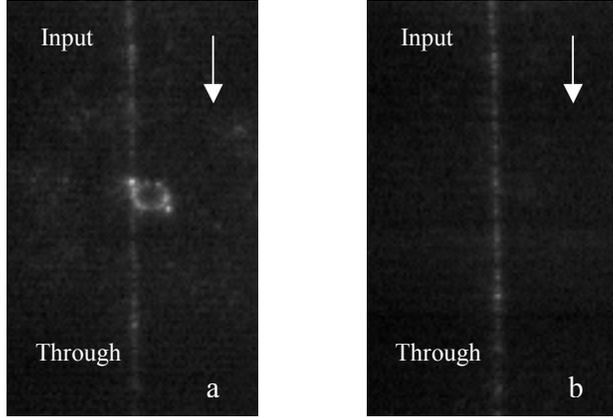
Fig.4 Images obtained by an IR camera of a MR around a wavelength of 1549 nm; a: on-resonance, b: off-resonance
