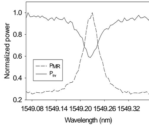
Fig. 6: Cavity power,  $P_{MR}$  (peak) from direct measurement and through port power,  $P_{thr}$  (dip) from indirect measurement
