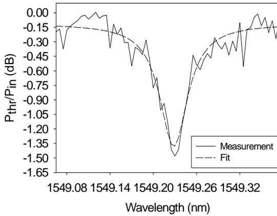
Fig.5: The through port power of a MR obtained by direct measurements after correction for the straight waveguide loss
