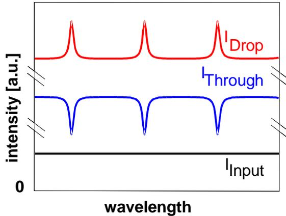
Fig.2: Spectral response of a microring resonator as a function of wavelength
