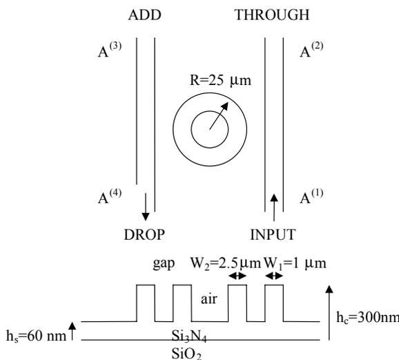
Fig.1: Top view and cross section of a microring resonator with laterally coupled waveguides
