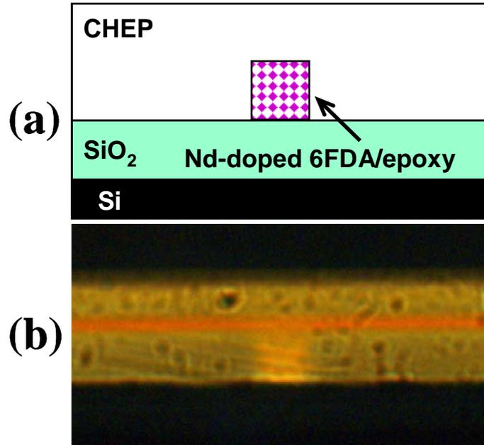
Fig. 1. (a) Geometry of the Nd<sup>3+</sup> doped polymer channel waveguides and (b) optical microscope picture of a channel waveguide cross section
