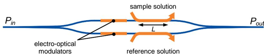
Figure 1. Top-view of a classical “straight” IO-MZI.
