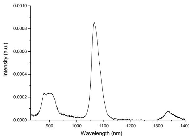
Fig. 1 Room temperature spontaneous emission of the Nd(TTA)<sub>3</sub>phen doped 6-FDA epoxy film pumped by Ti:Sapphire laser at 800nm.
