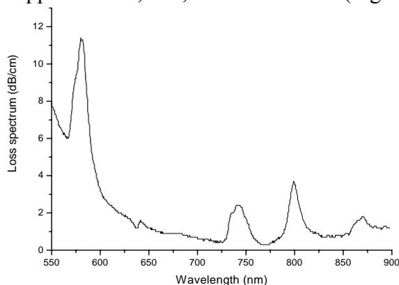
Fig. 3 Loss spectrum of the Nd(TTA)<sub>3</sub>phen doped 6-FDA epoxy channel waveguide.
