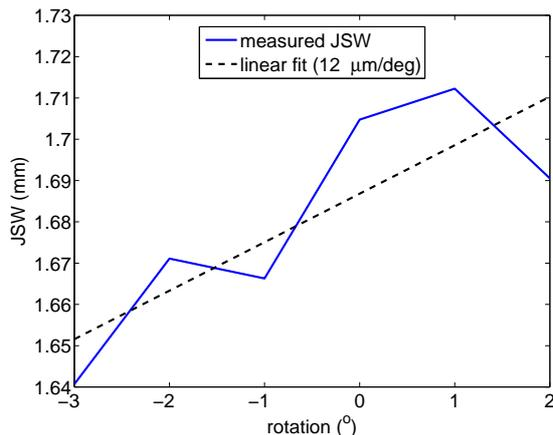
Figure 6: JSW as function of rotation around the X-axis for a skeleton
