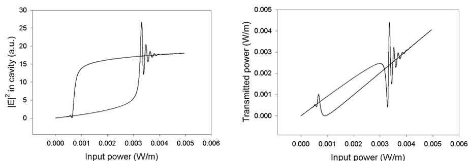
Figure 4: Hysteresis loops of intensity in cavity (left) and transmitted power (right) vs. input power.
