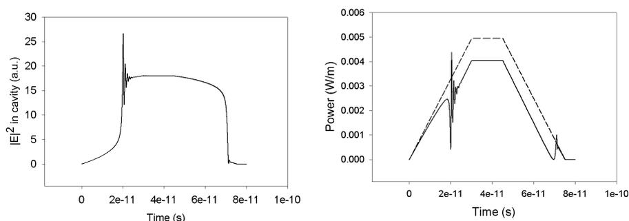
Figure 3: Left: Intensity in the cavity vs. time. Right: Input (dashed) and transmitted (solid) power vs. time.
