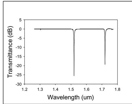
Figure 2: Transmission spectrum of notch filter
