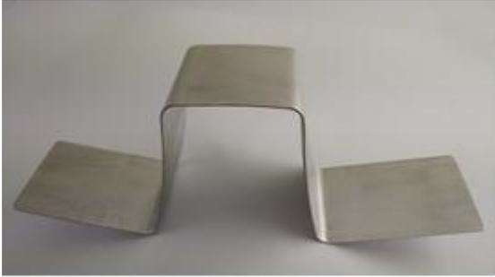
**Fig. 3** U-bend test part of AA6016 sheet material
