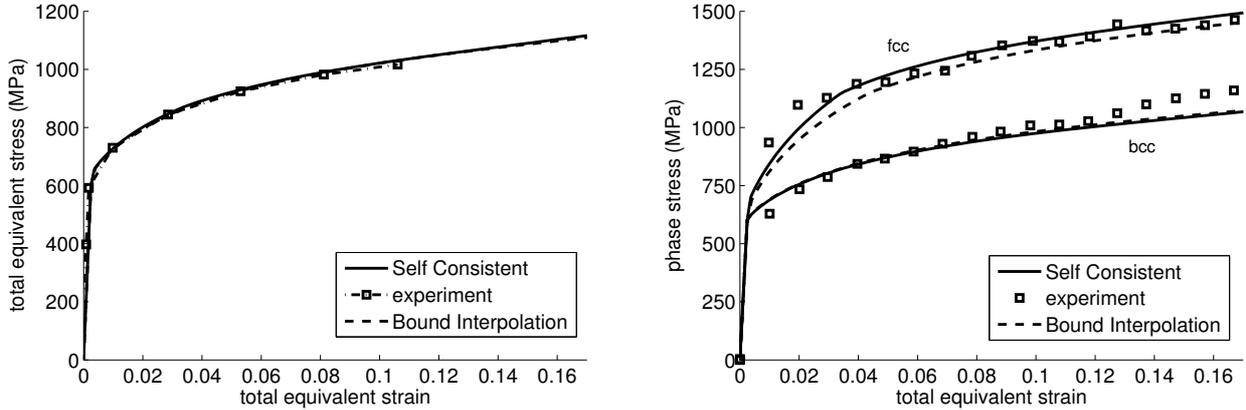
**FIGURE 1.** a) Overall stress as a function of overall strain, b) Stress in the phases as a function of overall strain
