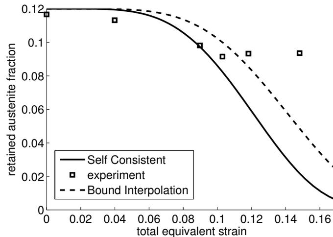
**FIGURE 2.** Fraction retained austenite as a function of overall strain
