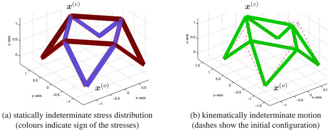
**Figure 2.** System with 12 rigid trusses, supported in the  $z = 0$  plane and connected in the  $z = 1$  plane.
