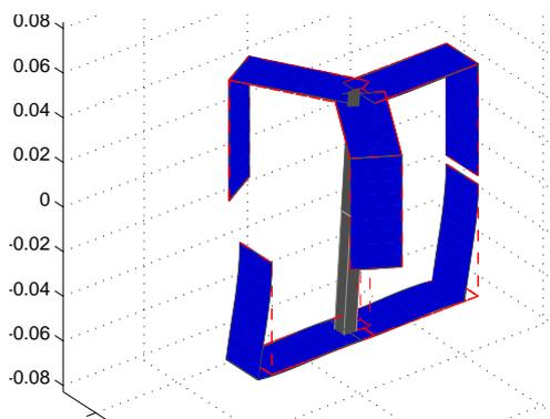
(a) Kinematically indeterminate motion
