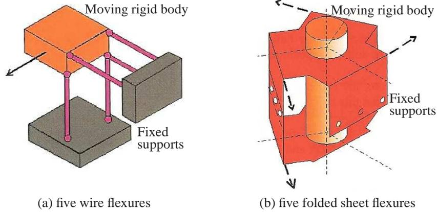
**Figure 3.** Two concepts for a one degree-of-freedom (1-DOF) straight guiding mechanism (reprinted from [8]). In (a) the solid arrow indicates the free movement. In (b) the cylinder represents the moving part. The supports are at the holes. The dashed arrows indicate directions of constraint movements.
