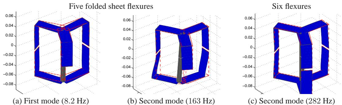
**Figure 6.** First and second mode shapes of the straight guiding mechanisms with five folded sheet flexures and the overconstraint design with six folded sheet flexures.
