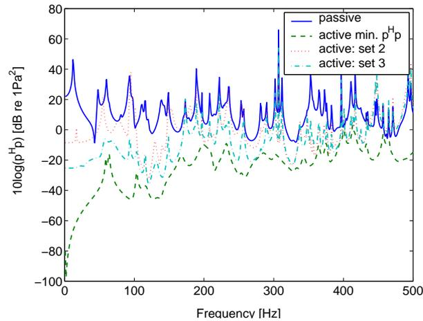
Figure 7: Active response with structural sensors (sensor set 2 and 3)
