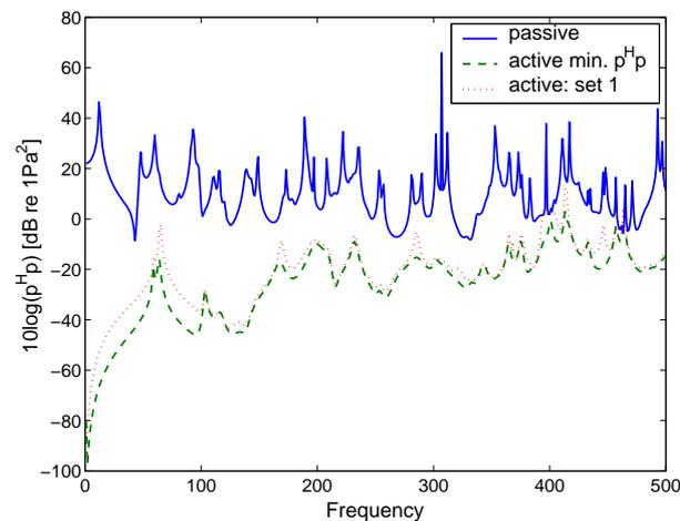
Figure 6: Active response with pressure sensors (sensor set 1)
