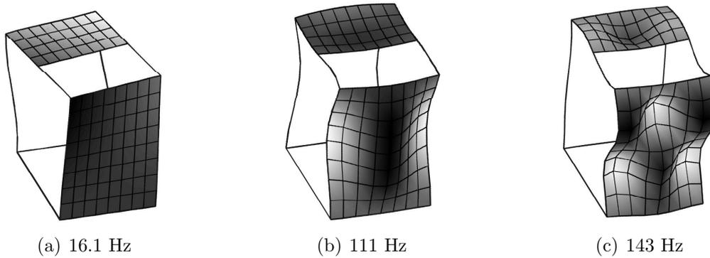
Figure 2: Some structural modes of the receiver with corresponding eigenfrequency
