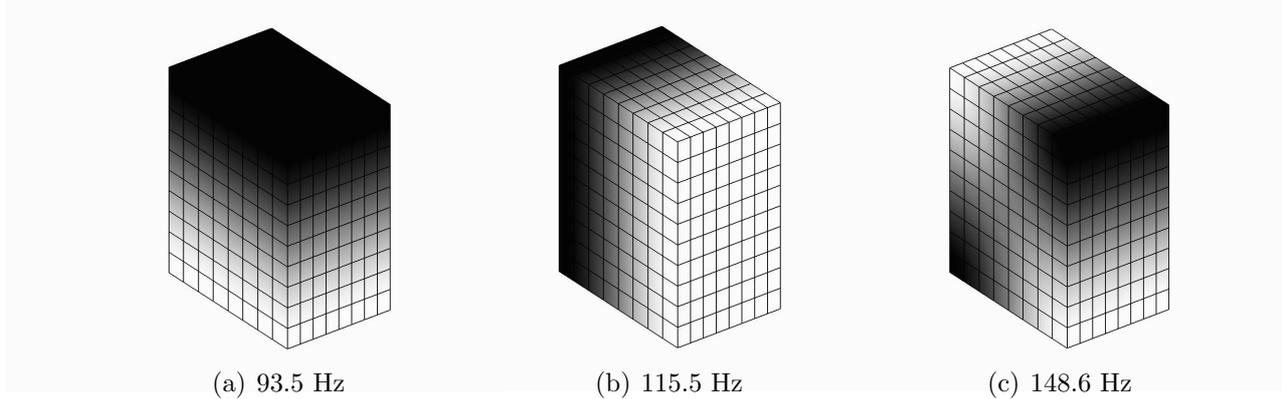
Figure 3: The pressure distribution of the 2<sup>nd</sup>, 3<sup>rd</sup> and 4<sup>th</sup> acoustic mode of the cavity
