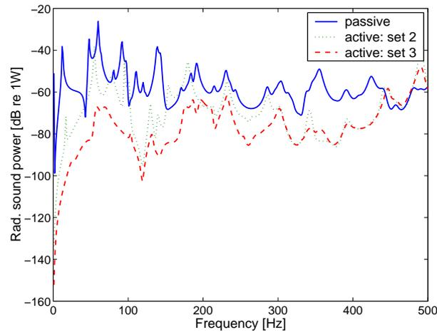
Figure 5: Active response with velocity sensors
