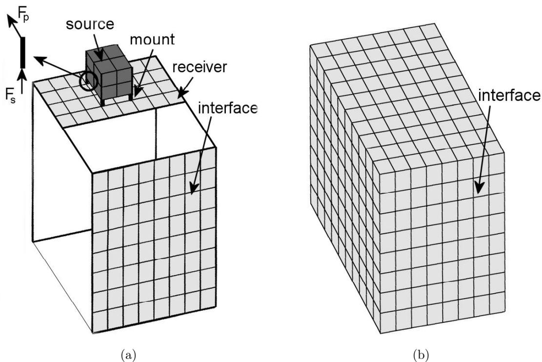
Figure 1: FEM-mesh of the structural part and acoustical part of the model.
