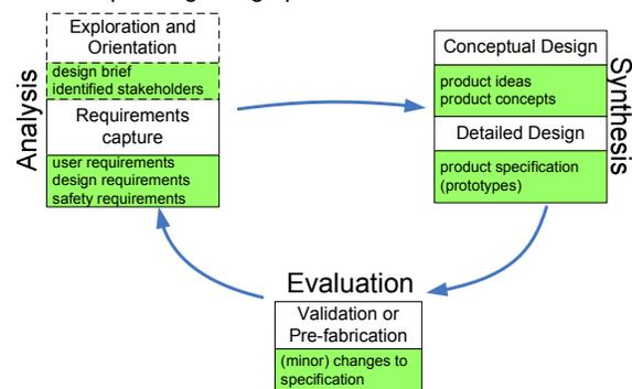
Figure 2 A representation of the design phases within a process loop of *analysis, synthesis and evaluation*; the green boxes show the outputs of the relevant phase.
