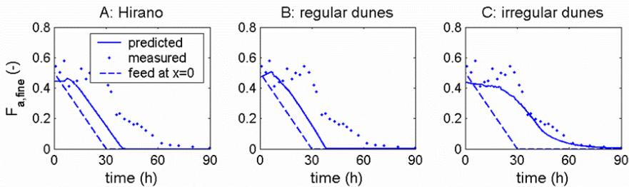
Figure 3. Volume fraction content of fines in bed load transport at the downstream end of the flume.
