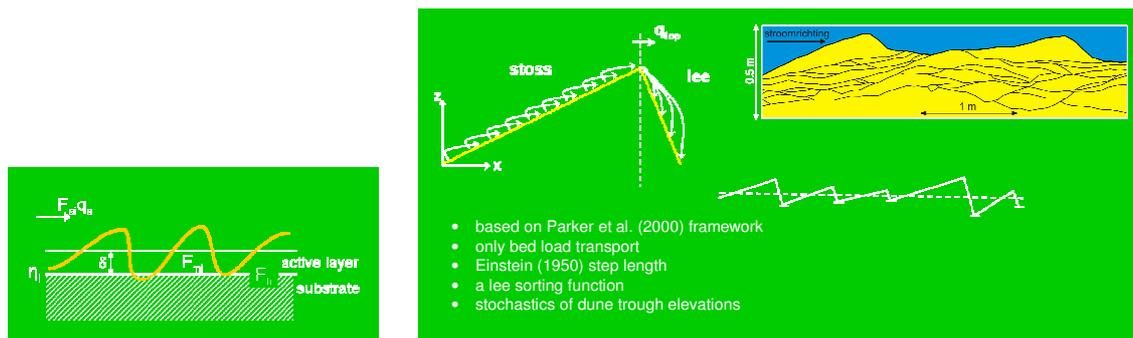
Figure 1. (a) The Hirano (1971) active layer model, and (b) The Blom & Parker (2004) probabilistic sediment continuity model for conditions with dunes.
