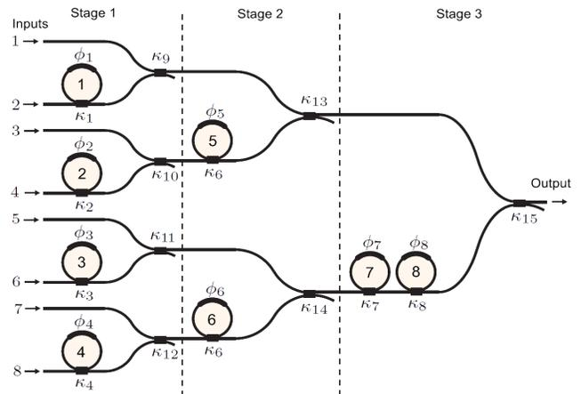
Figure 1. Schematic layout of the 8x1 OBFN
