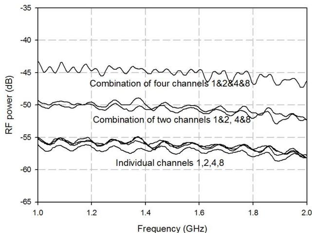
Figure 4. Measurement results of the RF-to-RF power response when of one (*bottom*), two (*middle*) and four RF inputs (*top*) are connected to the OBFN. The 6 dB increase at each doubling of the number of inputs demonstrates the OBFN coherent combining capability.
