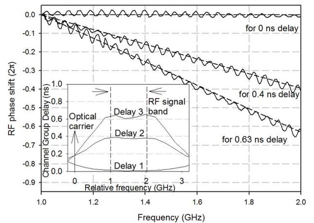
Figure 3. Measurement results of the RF-to-RF phase response of one OBFN channel, for three different delay settings. The minimum delay setting is used as reference 0 ns delay. The dashed lines indicate the ideal linear phase responses.
