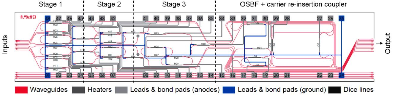
Figure 2. Mask layout of FLY 8x1 OBFN chip
