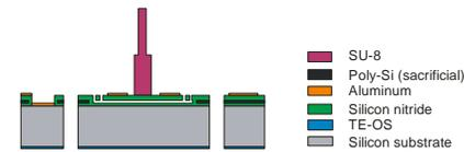
Figure 3. Schematic of the MEMS-based, artificial hair sensor
