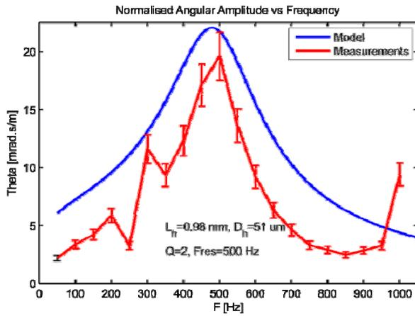
Measured and predicted sensitivity of artificial hair-sensors as a function of frequency.
