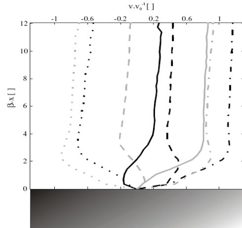
Measured sinusoidal flow-profile over a MEMS structure
