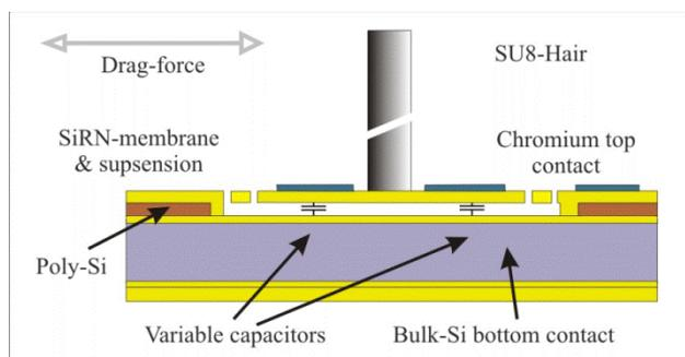
Schematic representation of an artificial hair-sensor
