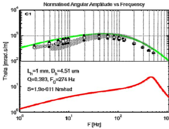
Comparison between cricket and MEMS hair-sensor deflections as a function of frequency.
