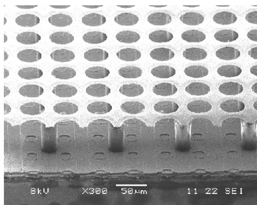
Figure 1. SEM picture of the detector, a punctured metal film placed over a CMOS chip is supported by insulating SU-8 or KMPR pillars.
