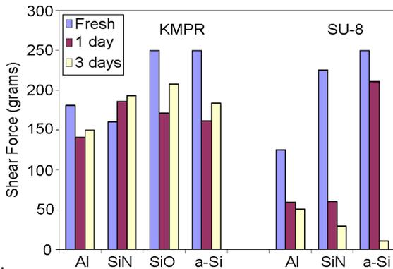
Figure 5. Adhesion strength of SU-8 and KMPR on different substrate materials; before humidity exposure (fresh) and after exposure to 95% relative humidity during one or three days.
