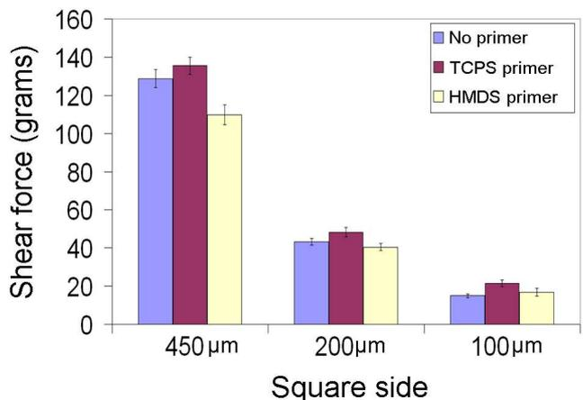
Figure 3. Adhesion of SU-8 on aluminum substrate for different primer treatments and different square sizes.
