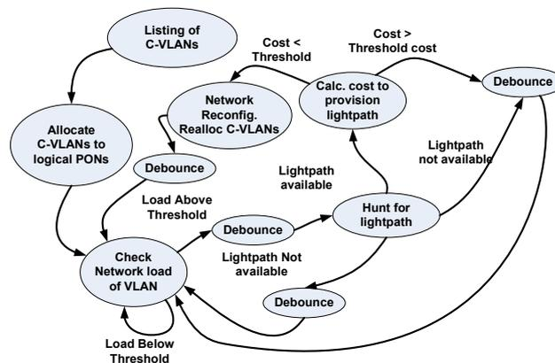
Figure 2: State diagram for C-VLAN allocation
