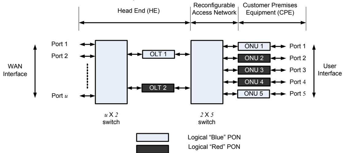
Figure 1: Network view as a two stage switch
