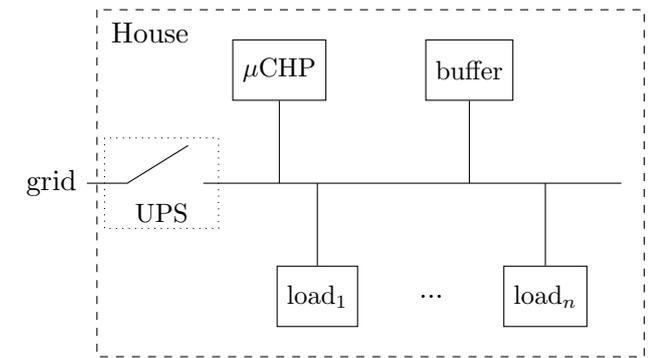
(a) Schematic of the electrical architecture of a house with islanding possibilities
