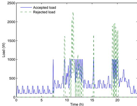
Fig. 4. Electricity demand cut off at 1kW
