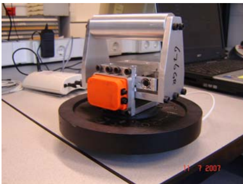
Figure 1. Experimental setup of a handle connected to a mass load, with 3D inertial and force/moment sensors.
