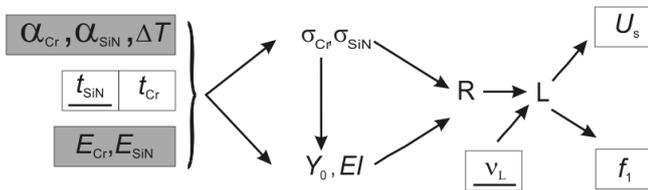
**Figure 2. Calculation strategy: Grey boxed values are fixed material properties. Underlined boxed values were chosen. Cr thickness was varied to find an optimum design.**
