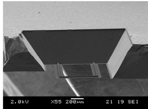
**Fig. 2** Free hanging U-shaped silicon nitride channel.
