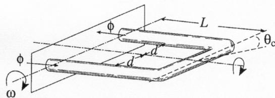
**Fig. 1** U-shaped Coriolis sensor ( $\theta_c$  is the deformation due to torsion, caused by the Coriolis force) [1].
