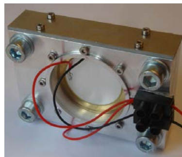
Fig. 7. Photograph of SJA used in test set-up
