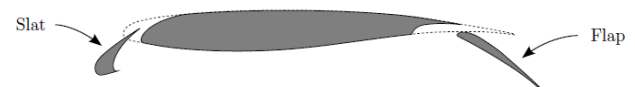
Fig. 1. Section of a high-lift wing section with a leading-edge slat and single-slotted trailing-edge flap (adapted from [1])
