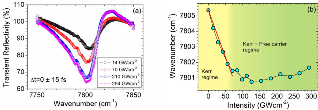
**Fig. 1** (a) Reflectivity vs. frequency at different pump intensities. (b) Cavity resonance frequency vs. pump intensity at zero delay between pump and probe.
