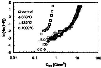
Fig 1: Weibull plot of  $Q_{bd}$  as a function of anneal temperature. Electrons are injected from the bottom electrode. A constant current density of  $2.5 \text{ mA/cm}^2$  was applied to capacitor structures with an area of  $1 \cdot 10^{-4} \text{ cm}^2$ .
