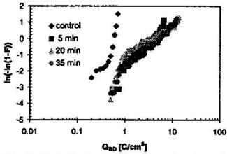
Fig 4: Weibull plot of  $Q_{bd}$  as a function of anneal time. Electrons are injected from the bottom electrode. A constant current density of  $2.5 \text{ mA/cm}^2$  was applied to capacitor structures with an area of  $1 \cdot 10^{-4} \text{ cm}^2$ .
