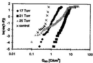
Fig 7: Weibull plot of  $Q_{bd}$  as a function of anneal pressure. Electrons are injected from the bottom electrode. A constant current density of  $2.5 \text{ mA/cm}^2$  was applied to capacitor structures with an area of  $1 \cdot 10^{-4} \text{ cm}^2$ .
