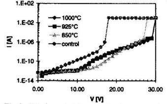
Fig 3: I-V characteristics for the three anneal temperatures and the control oxide. The dielectric thickness of all capacitor structures was 25 nm.
