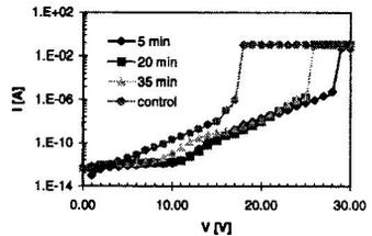
Fig 6: I-V characteristics for different anneal times and the control oxide. The dielectric thickness of all capacitor structures was 25 nm.
