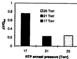
Fig 8:  $\Delta V/Q_{bd}$  as a function of anneal pressure. The control oxide is not shown as a consequence of the scalability ( $\Delta V/Q_{bd}=5.5$ ).
