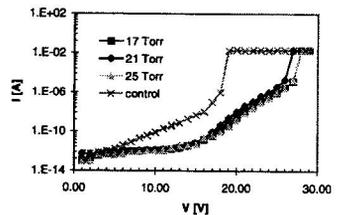
Fig 9: I-V characteristics for different anneal pressures and the control oxide. The dielectric thickness of all capacitor structures was 25 nm.
