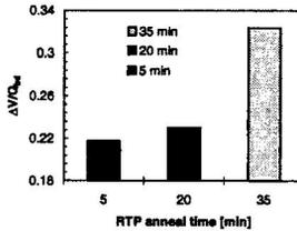
Fig 5:  $\Delta V/Q_{bd}$  as a function of anneal time. The control oxide is not shown as a consequence of the scalability ( $\Delta V/Q_{bd}=5.5$ ).
