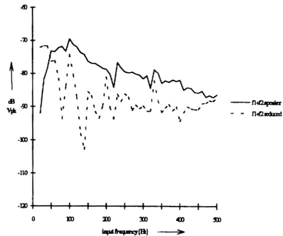
Fig. 4. Frequency  $f_1+f_2$  from the speaker with and without distortion reduction circuit
