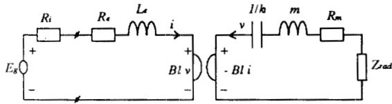
Fig. 1. Lumped parameter equivalent circuit of an electrodynamic loudspeaker
