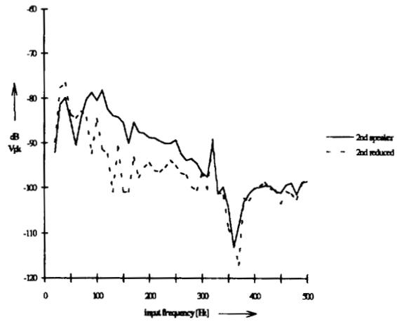
Fig. 3. Second harmonic of the loudspeaker with and without distortion reduction circuit
