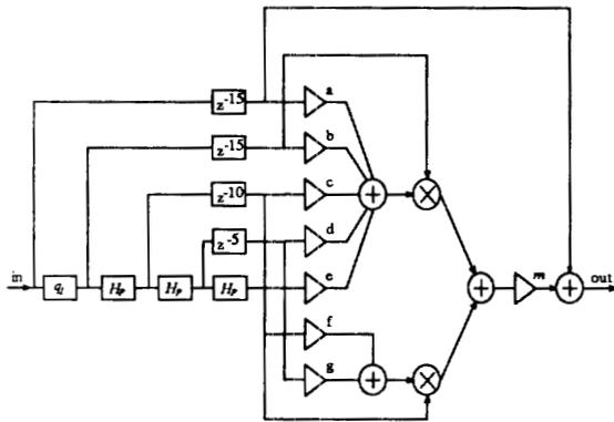
Fig. 2. Second order distortion reduction circuit
