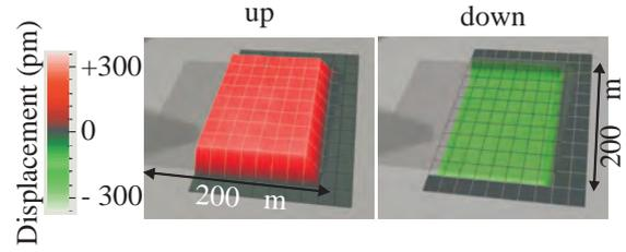
Figure 4: Scanning laser-Doppler vibrometer measurements of a 250 nm thick PbZr<sub>0.52</sub>Ti<sub>0.48</sub>O<sub>3</sub> film. By applying an 8 kHz and 6 V peak to peak ac-voltage and measuring the maximum displacement of the top electrode, the piezoelectric coefficient ( $d_{33,f}$ ) was measured.
