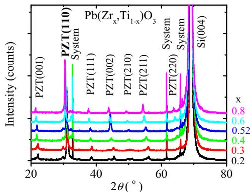
Figure 7: Measured x-ray diffraction patterns of the pulsed laser deposited  $\text{Pb}(\text{Zr}_x\text{Ti}_{1-x})\text{O}_3$  thin films, plotted for different compositions. The PZT films display a preferred (110) orientation.
