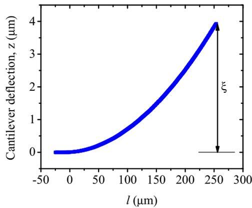
Figure 6: Profile of the cantilever deflection after the deposition of PZT ( $x=0.52$ ). A Maximum upward displacement  $\xi$  of the free end of the cantilever of almost  $4 \mu\text{m}$  can be clearly seen from the image at  $l=250 \mu\text{m}$ .
