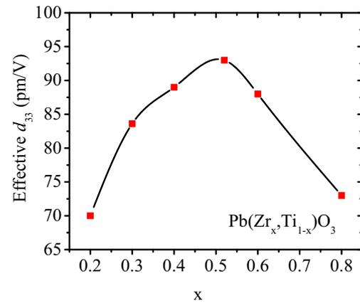
Figure 8: The effective longitudinal piezoelectric coefficient ( $d_{33,f}$ ) of different compositions. Based on our measurements we find the maximum value of  $d_{33,f}$  for  $x=0.52$ . The lines are guides to the eye.
