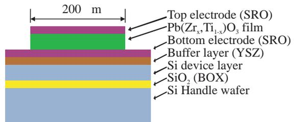
Figure 2: Illustration of a PZT thin film between top and bottom electrodes. PZT capacitors are needed to measure the longitudinal piezoelectric coefficient. The thickness of the PZT film is 250 nm. The thickness of both the SRO electrodes and YSZ is 100 nm each.
