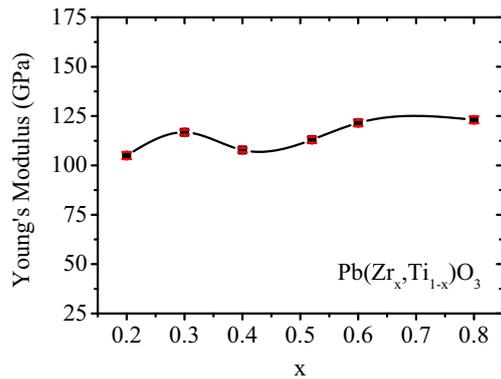
Figure 10: Zr/Ti composition dependence of Young's modulus of the PZT thin films plotted as a function of Zr content ( $x$ ) in  $\text{Pb}(\text{Zr}_x\text{Ti}_{1-x})\text{O}_3$  thin films. The lines are guides to the eye.
