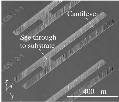
Figure 3: Scanning electron micrograph of the fabricated cantilevers. Cantilevers were fabricated from a 3 μm thick silicon device layer. Length varies from 250 μm to 350 μm in steps of 10 μm with a constant width of 30 μm.
