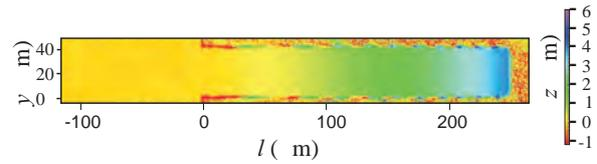
Figure 5: White light interferometry measurements of the static deflection of a 250 μm long cantilever after deposition of the PbZr<sub>0.52</sub>Ti<sub>0.48</sub>O<sub>3</sub> thin film. Length and width of the cantilever are represented by  $l$  and  $y$ . Parameter  $z$  represents the transverse deflection of the cantilever.
