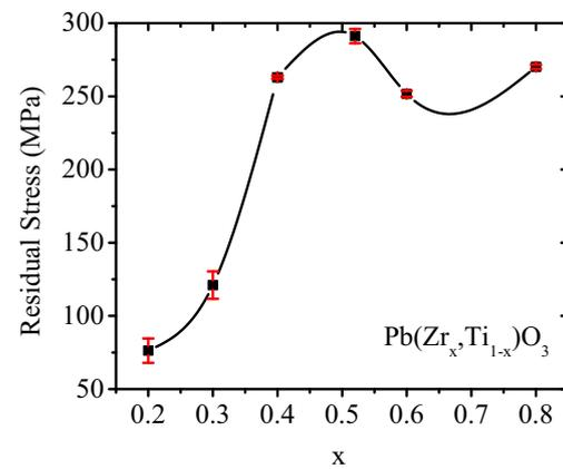
Figure 9: Compositional distribution of the residual stress in the PZT thin films. Residual stress in the PZT thin film increases with the increasing Zr content. The lines are guides to the eye.
