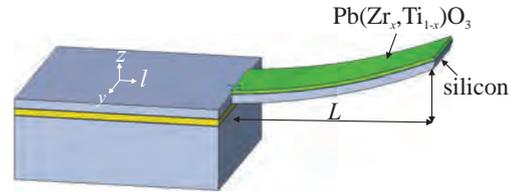
Figure 1: Schematic representation of a cantilever fabricated from a silicon on insulator wafers. The upward static deflection is due to the tensile residual stress in the PZT thin film that was deposited on the cantilever.
