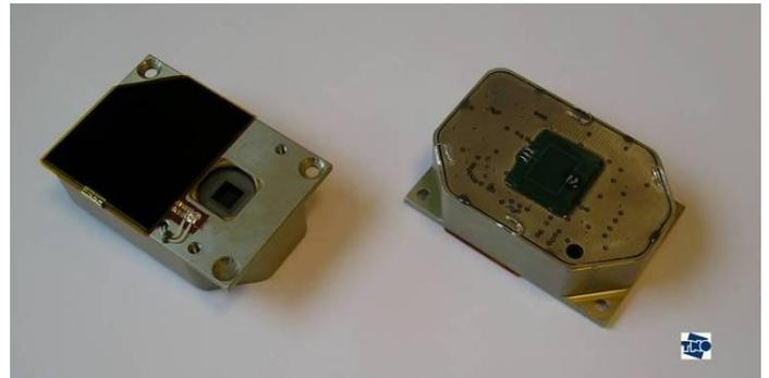
*Fig.1. Autonomous Wireless Sun Sensor build by TNO in the Netherlands.*
