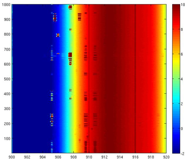
Fig.5 Waterfall plot of the one of the passes of Delfi-C3 at the WSRT with the telescopes positioned along the orbit direction.
