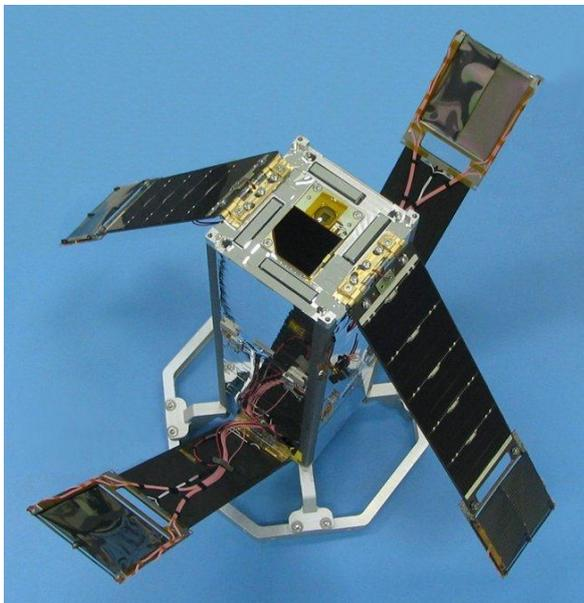
Fig. 4. Stripped layout of the Delfi-C3 satellite.
