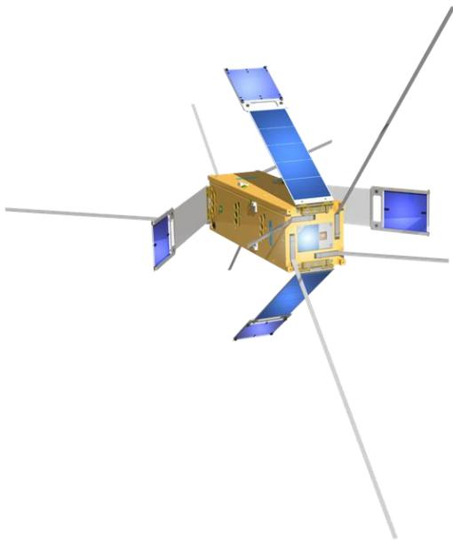
*Fig.2. Delfi-C3 satellite with two AWSS mounted on both the small faces of the satellite.*
