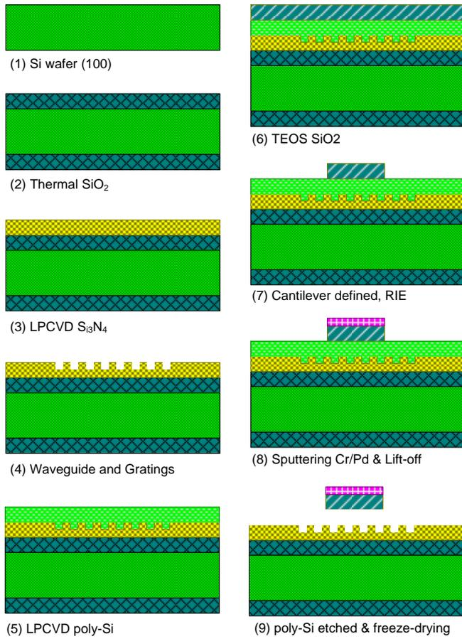
Fig.2. Process flow chart of fabrication of an integrated mechano-optical sensing device
