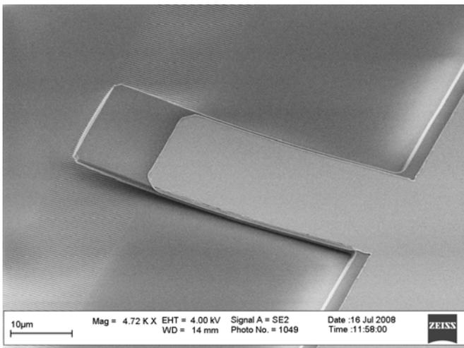
Fig. 5. SEM image of the fabricated device with a suspended cantilever above a 490 nm periodic grating
