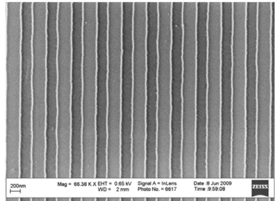
Fig.3. SEM image of a grating with period of 490 nm, fabricated by laser interference lithography (LIL)
