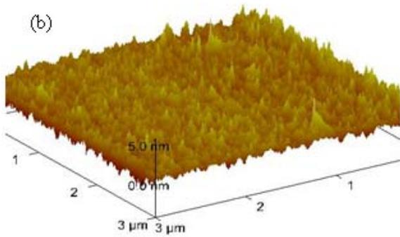
Fig.4. AFM topographic images of  $\text{Si}_3\text{N}_4$  surface roughness, affected by (a)  $\text{SF}_6$  dry-etching ( $R_q=25.6\text{nm}$ ) and (b) TMAH wet-etching ( $R_q=0.46\text{ nm}$ )
