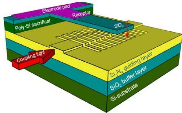
Fig. 1. The grating waveguide-cantilever device
