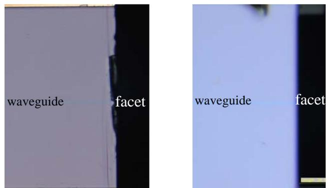
Fig.7. Optical microscopic images of facets: (left) a rough and cracked cleaved facet and (right) a smooth facet obtained by the new technique
