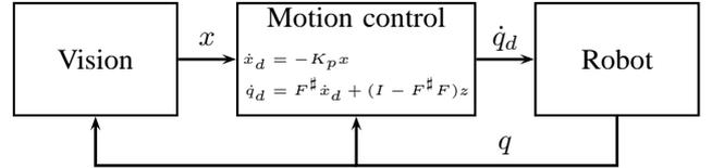
Fig. 2. Overview of the control scheme.
