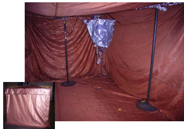
Figure 3: A Tuneable Intrinsic Reverberation Chamber, lower left outside, right inside
