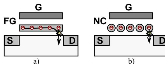
Fig. 1. Possible leakage path in the tunnel oxide in non-volatile memory cell with continuous floating gate (a) and with nano-crystals (b).
