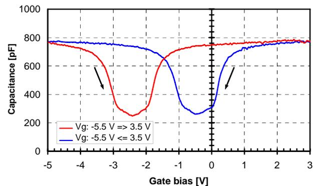
Fig. 8. QS-CV hysteresis curves obtained during programming and erasing cycles for MOS structures with encapsulated silicon nano-crystals. Applied gate-substrate voltages: Vg prog = 3.5 V and Vg erase = -5.5 V.
