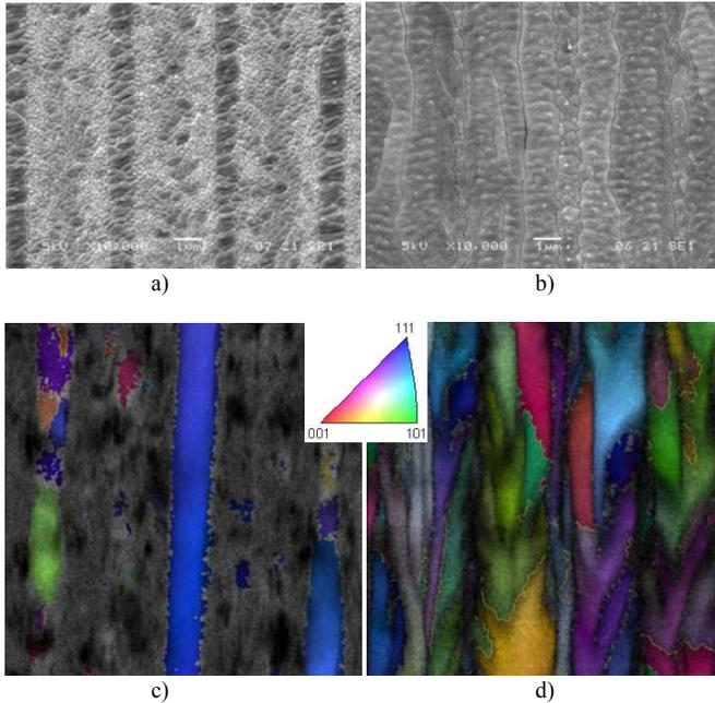
Fig. 4. SEM images and inverse pole figure (IPF) maps of  $\alpha$ -Si films crystallized with energy densities 0.6 J/cm<sup>2</sup> (a, c) and 1.0 J/cm<sup>2</sup> (b, d) at 98% laser beam overlapping.
