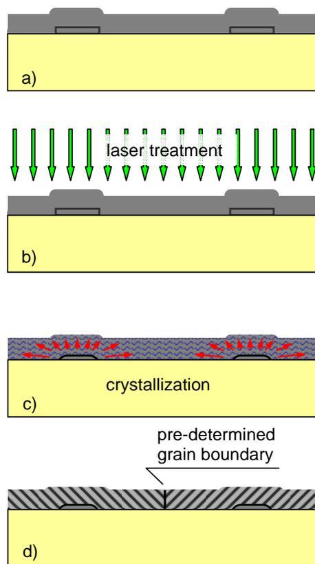
Fig. 3. Crystallization process in silicon film with preformed lines (a) film formation, (b) laser treatment, melting of the silicon film, (c) crystallization process – super lateral growth, (d) finally crystallized film with predefined grain boundaries.
