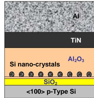
Fig. 7. The schematic cross-section of the multilayer structure with encapsulated silicon nano-crystals.
