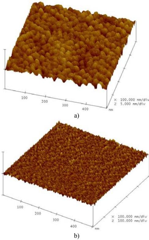
Fig. 6. AFM images of oxidized Si-NC layers deposited at 325°C from disilane at 10 mbar (a) and from trisilane at 1 mbar (b). To enable the observation of the nano-crystals, no upper protection layer was deposited.
