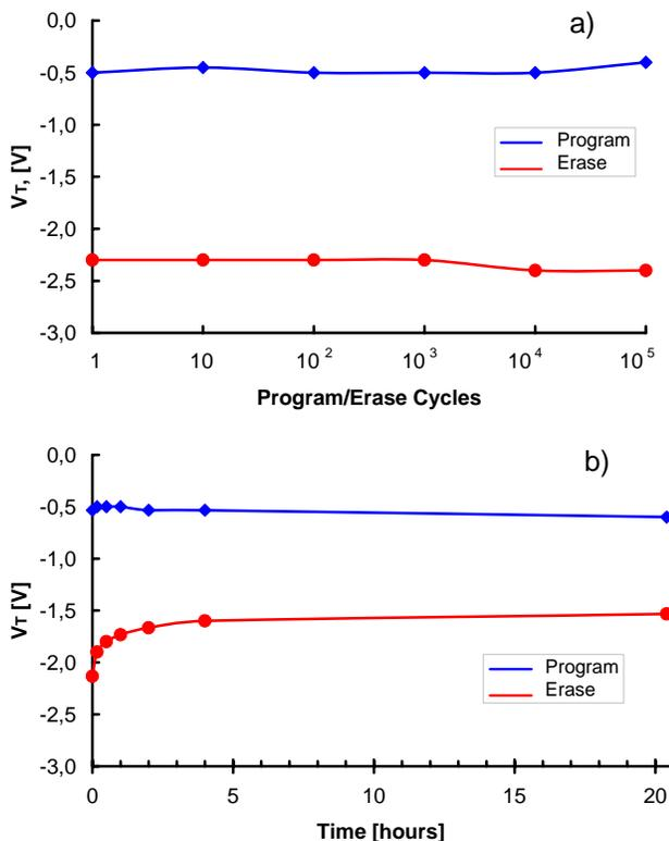
Fig. 9. Endurance (a) and retention (b) measurements of MOS structures with encapsulated silicon nano-crystals.
