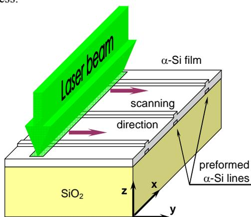
Fig. 2. The laser crystallization process of a silicon film with preformed lines.
