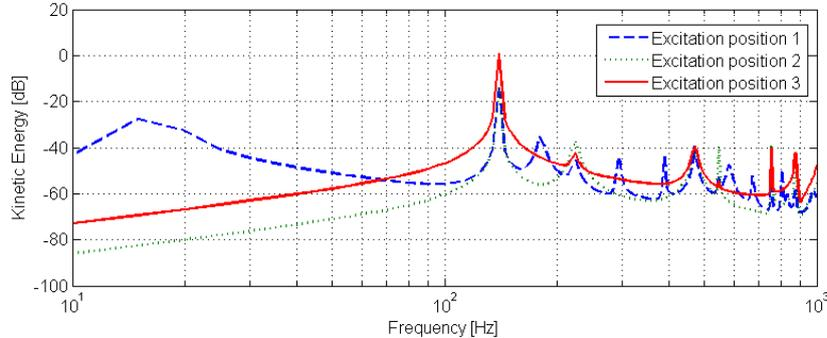
Figure 4 - Simulation of the kinetic energy response of the panel with various excitation positions
