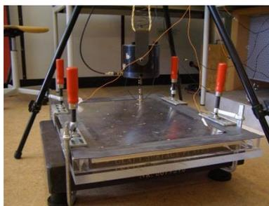
Figure 1 - Mode shapes and resonant frequencies measurement of the panel attached to the cabinet
