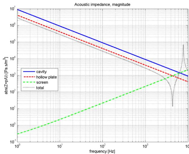
Figure 2 – Lumped acoustic impedance load as seen by the back of the radiating structure.
