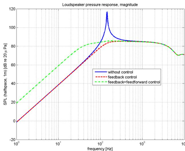
Figure 3 – Sound pressure level at 1m distance, 1W nominal input power, half-space radiation
