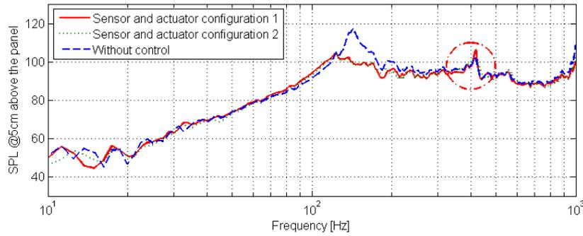
**Figure 5 - Sound pressure level (SPL) response of the flat loudspeaker with various sensor-actuator configurations**
