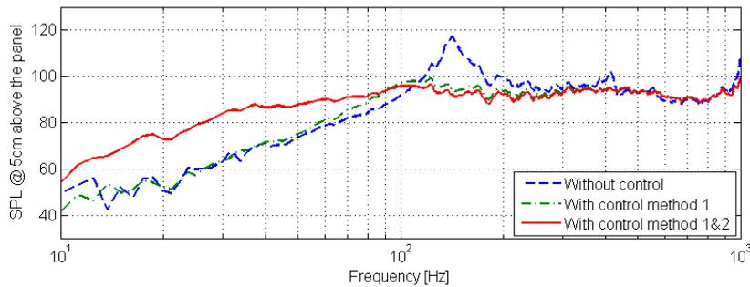
**Figure 6 - SPL response of the flat loudspeaker with control sensor-actuator configuration 3**
