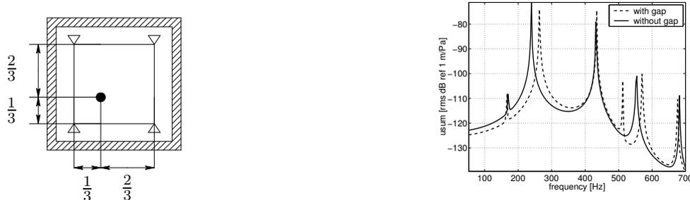
Figure 7: Source position (left) and vibration response of liner (right)
