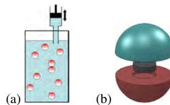
Figure 2: (a) Schematic drawing of the experimental setup. Shown are the beaker, which contains the liquid with the milli-magnetic particles, and the inlet to which an agitation pump can be connected. (b) Exploded view of a milli-magnetic particle. Shown are the neodymium magnet and the 3D-printed plastic encapsulation, which consist of two half-spheres; their difference in color allows to identify the 'North' and 'South' pole of the particle.
