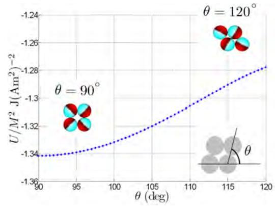
Figure 5: *The in-plane trajectory in the energy landscape of a 4-dipole system. The energy is plotted against  $\theta$ , which is defined in the lower right inset. The magnetic configurations after energy minimization for  $\theta = 90^\circ$  and  $\theta = 120^\circ$  are also shown.*
