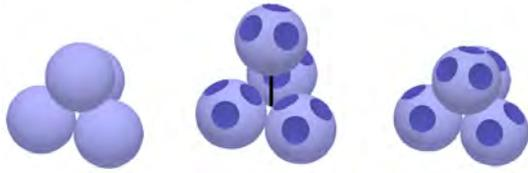
Figure 7: Illustration of a shape modification. The unmodified particles (left drawing) can be indented to allow a closer packing of the spheres (right drawing). The exploded view (center drawing) shows the indentations and the vertical trajectory (line) of the top particle.
