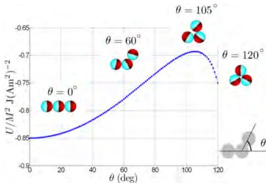
Figure 4: *Trajectory in the energy landscape of a 3-dipole system; the energy is plotted against  $\theta$ , which is defined in the lower right. The insets show the configuration of the particles for various  $\theta$ , after minimization of the energy.*
