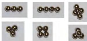
Figure 1: Photographs of simple configurations of toy magnets ('neocubes') with a diameter of 4 mm. All the configurations are stable, except for the two rightmost configurations; when the magnets are forced in one of these meta-stable configurations, they readily rearrange when touched.
