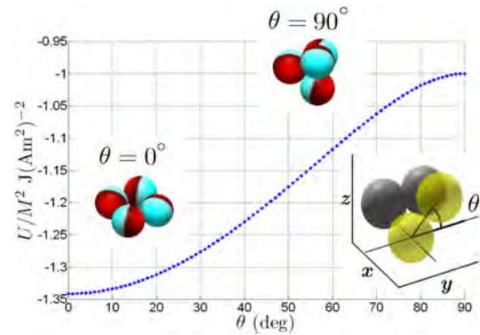
Figure 6: *The out-of-plane trajectory in the energy landscape of a 4-dipole system. The energy is plotted against  $\theta$ , which is defined in the lower right inset. The magnetic configurations after energy minimization for  $\theta = 0^\circ$  and  $\theta = 90^\circ$  are also shown.*
