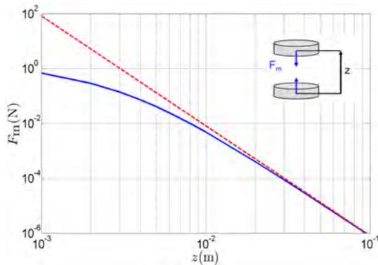
Figure 3: Force between two cylindrical magnets with a common axis, as a function of center to center separation. The cylinders have an axial magnetization and dimensions as listed in table 1. The exact solution [4] (solid line) and dipole approximation (dashed line) are shown.
