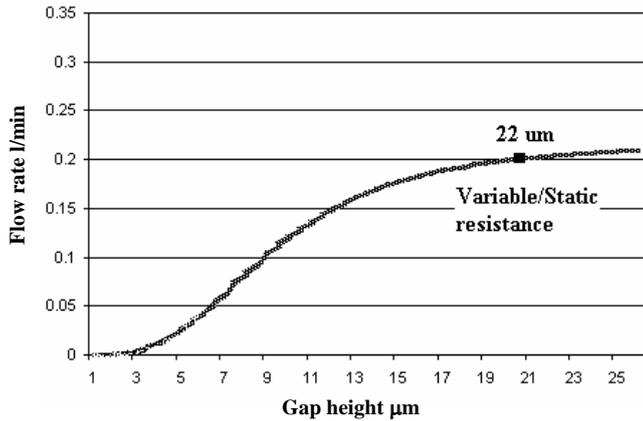
**Figure 3: variable resistance provides more linearity and less steep flow behavior**
