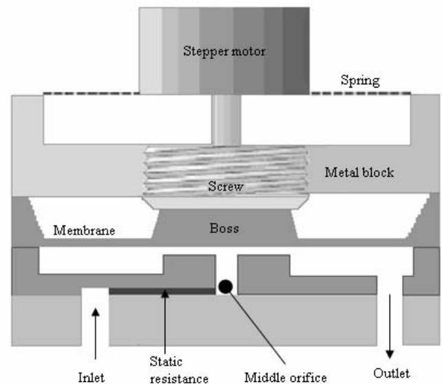
Figure 1: Schematic cross sectional view of the microvalve.
