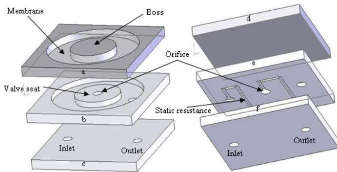
**Figure 5: Three dimensional view of microvalve with circular boss**
