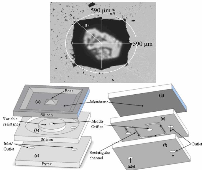
**Figure 4: Square boss with required size could not be realized with KOH time stop etching**
