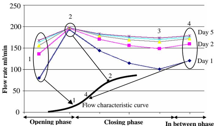
**Figure 9: Combined effect of Hysteresis in stepper motor, change in ambient conditions and wear in the screw threads cause high difference in flow rates.**
