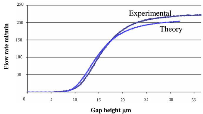
Figure 8: Experimental results are in accordance with the theory.
