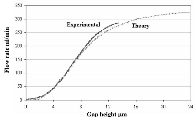
Figure 2: Flow reaches its maximum value at a gap height of 9  $\mu\text{m}$  instead of 22  $\mu\text{m}$  due to less static resistance available.
