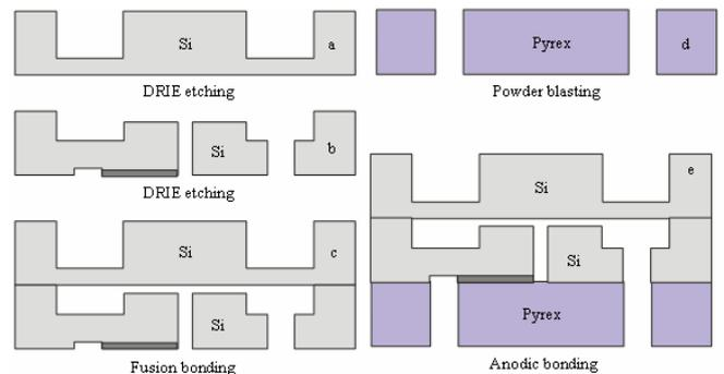
**Figure 6: Fabrication of micromachined part**
