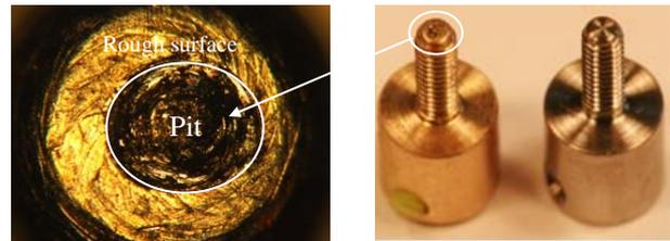
**Figure 10: A part of the brass screw was eroded**
