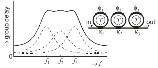
Figure 2. Theoretical group delay response of three cascaded ORR sections. The dashed lines represent the group delay responses of the individual sections. (Inset: cascade of three ORRs with round-trip delay  $T$ , additional round-trip phase-shifts  $\phi$  and power coupling coefficients  $\kappa$ .)
