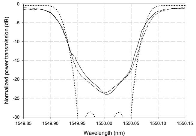
Figure 6. Measured normalized cross port power transmission of the OSBF chip. (The solid line shows the measured result. The dashed line is the simulated result for an ORR power coupling coefficient of 0.8, an MZI power coupling coefficient of 0.6, and an ORR roundtrip loss of 3 dB. The dotted line is the simulation for the same filter parameters but an ORR roundtrip loss of 0.082 dB.)
