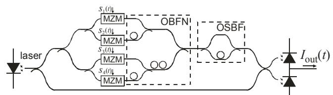
Figure 1. Schematic of the ring resonator-based optical beam forming system (MZM: Mach-Zehnder modulator, OBFN: optical beam forming network, OSBF: optical sideband filter).
