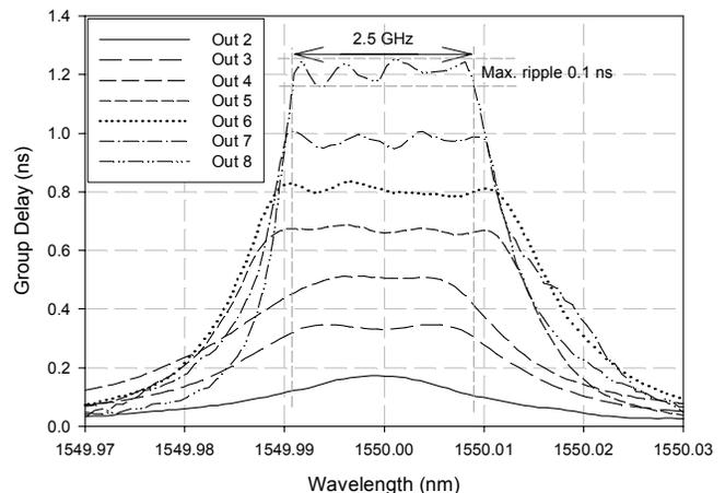
Figure 5. Measured group delay responses at different outputs of the 1×8 OBFN chip.
