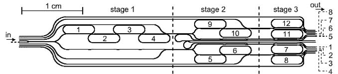
Figure 4. Waveguide structure of the 1×8 OBFN chip. The numbering of the rings and the outputs corresponds to the numbering in Fig. 3.
