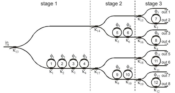
Figure 3. Binary tree-based  $1 \times 8$  optical beam forming network for a transmitter system, consisting of 12 ORRs and 7 tunable splitters.
